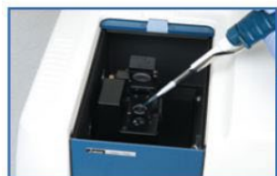
Step 1 Drop a sample on the cell.
