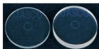
Dedicated disk cell for SAH-769 Optical pathlength : 1 mm (left), 0.2 mm (right) Sample volume : 5 \mu L (left), 0.6 \mu L (right)
