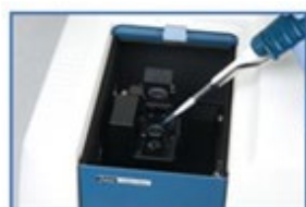
Step 1 Drop a sample on the cell.
