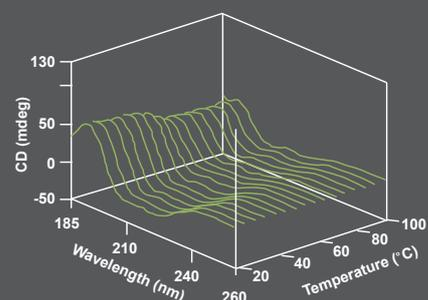
3D view of CD scans as a function of wavelength and temperature.
