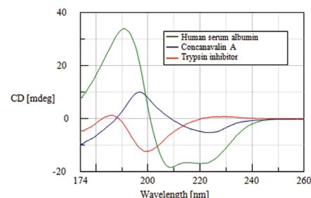
CD spectra of Human Serum Albumin (Helix rich), Concanavalin A (β-sheet rich) and Trypsin inhibitor (Random rich) in water with excellent signal to noise to 174 nm.
