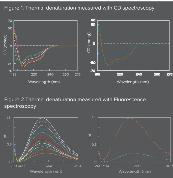
**Figure 1. Thermal denaturation measured with CD spectroscopy**
