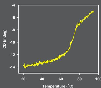
CD signal at 222 nm as a function of temperature.
