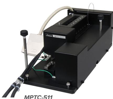
The MPTC accessories are designed to enable high sample throughput and productivity. The six-position holder for rectangular cells allows automated spectral scans and parallel thermal ramps on up to six samples at a time. Applicable measurement modes include spectral scans, thermal ramping at single or multiple wavelengths, and thermal ramplng with spectral scans at preset temperatures.
