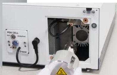
Front panel access for easy lamp replacement
