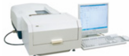
V-600 with the Absolute Reflectance Accessory
